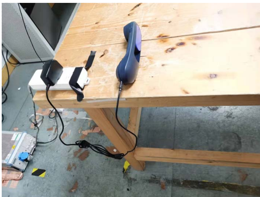
Photo of Power Line Conducted Emission Measurement - Side View
