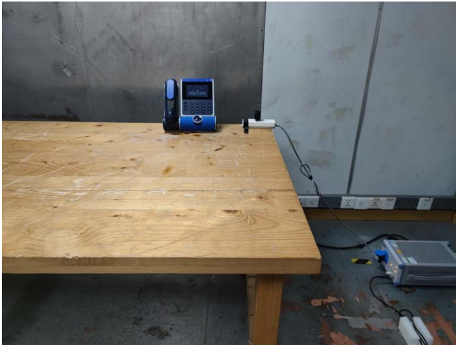
Photo of Power Line Conducted Emission Measurement - Front View Telephone Base Charging
