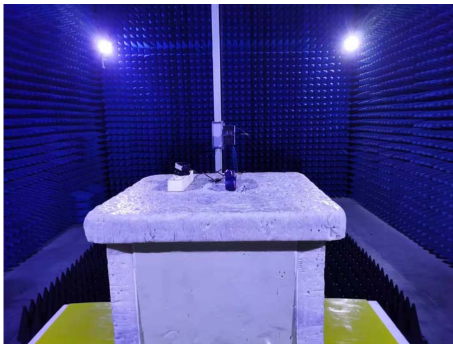
Photo of Radiated Emission Measurement Above 1GHz
