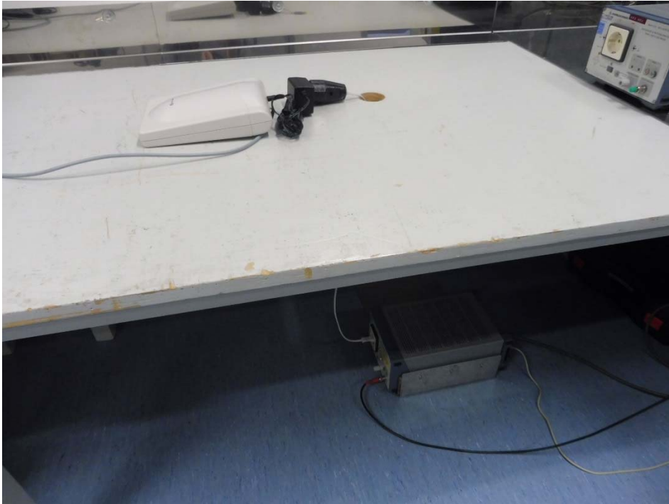
Photo 1: Conducted Emission Test
