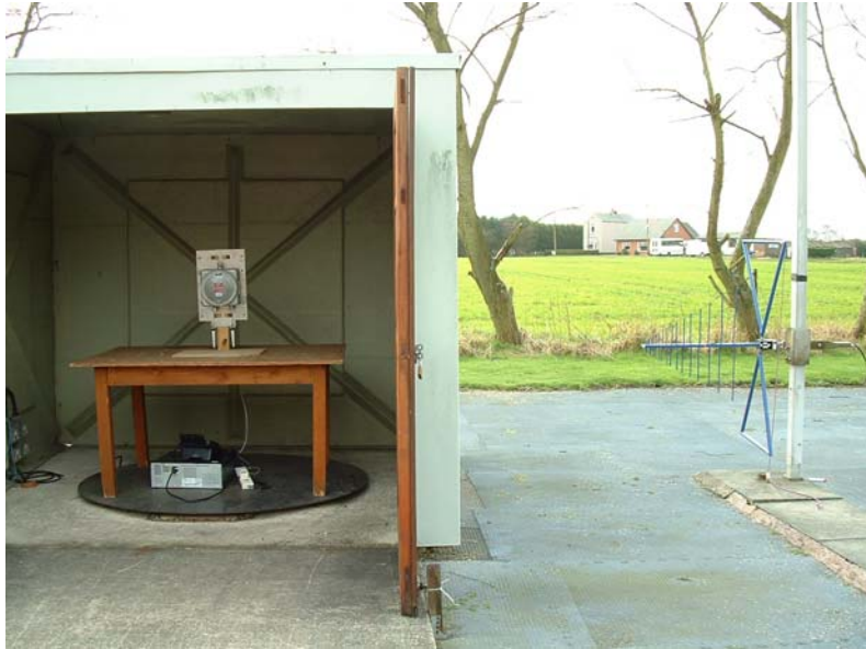
4070 IO Ex On Open Area Test Site
