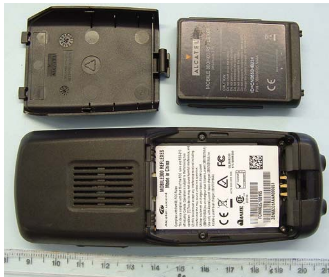
PHOTOGRAPH No. 5 MR300 REAR OVERVIEW COVER & BATTERY REMOVED
