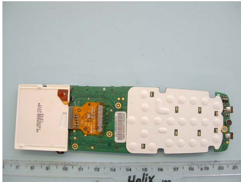
MR400 PCB KEYPAD SIDE LCD MOVED
