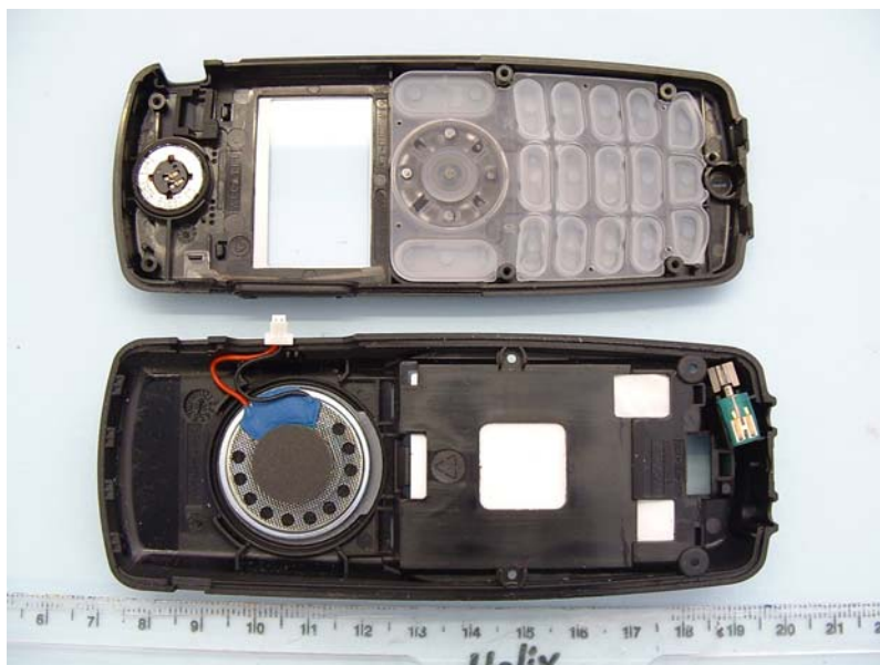
MR400 CASE INTERNAL VIEW PCB REMOVED
