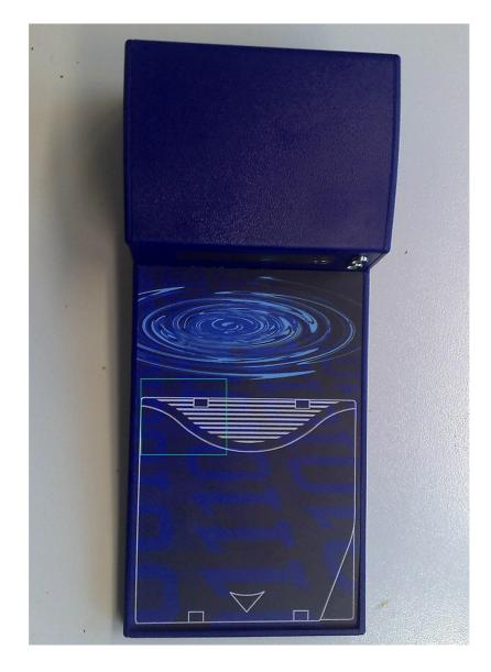
Hint: the reader generates a magnetic field with the frequency of 13.56MHz which is influenced by any electrically conductive material in close proximity to the antenna. A minimum of 10 cm is required to ensure that there will be no significant degradation of the performance in terms of read range and reliability.
