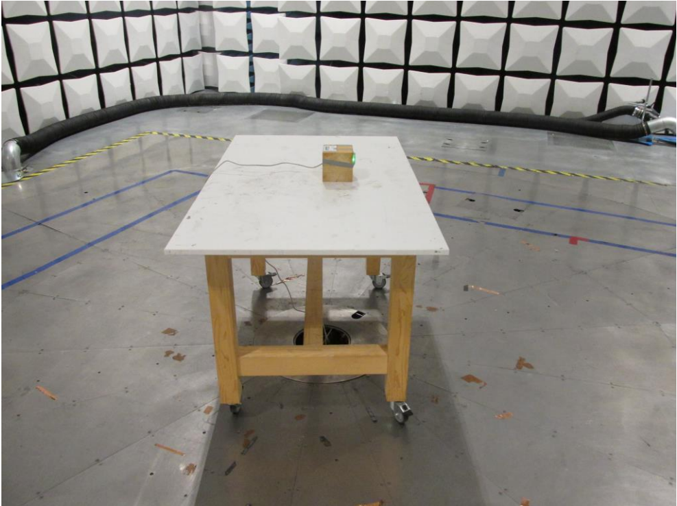
Figure 11 - Test setup for radiated emission
