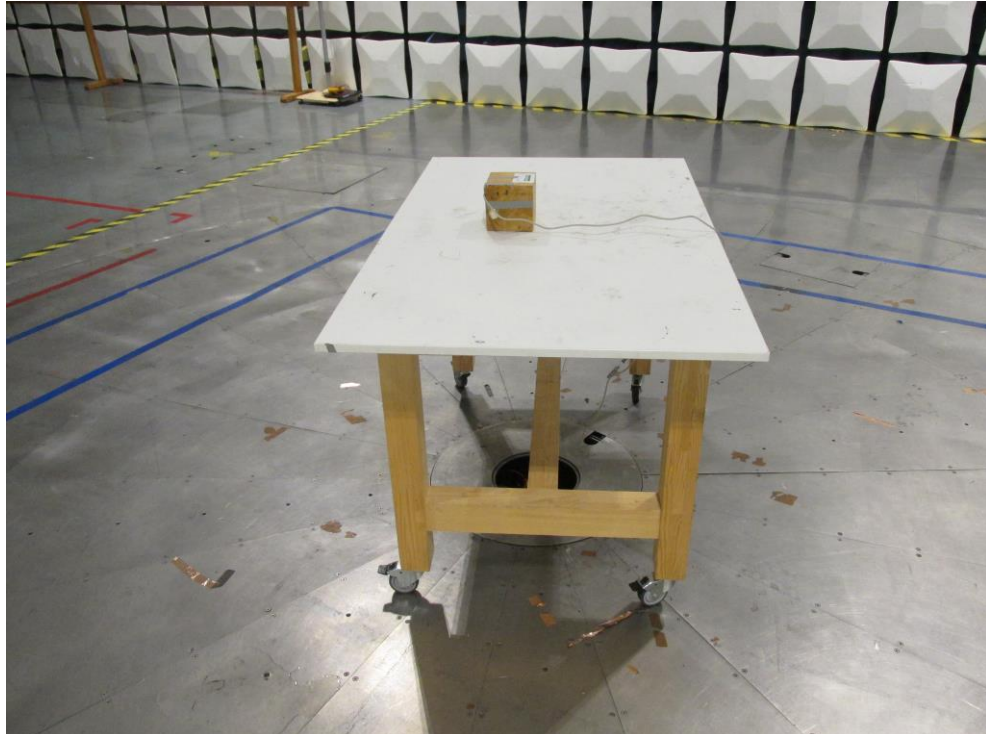
Figure 13 - Test setup for radiated emission
