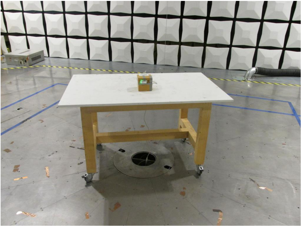
Figure 10 - Test setup for radiated emission
