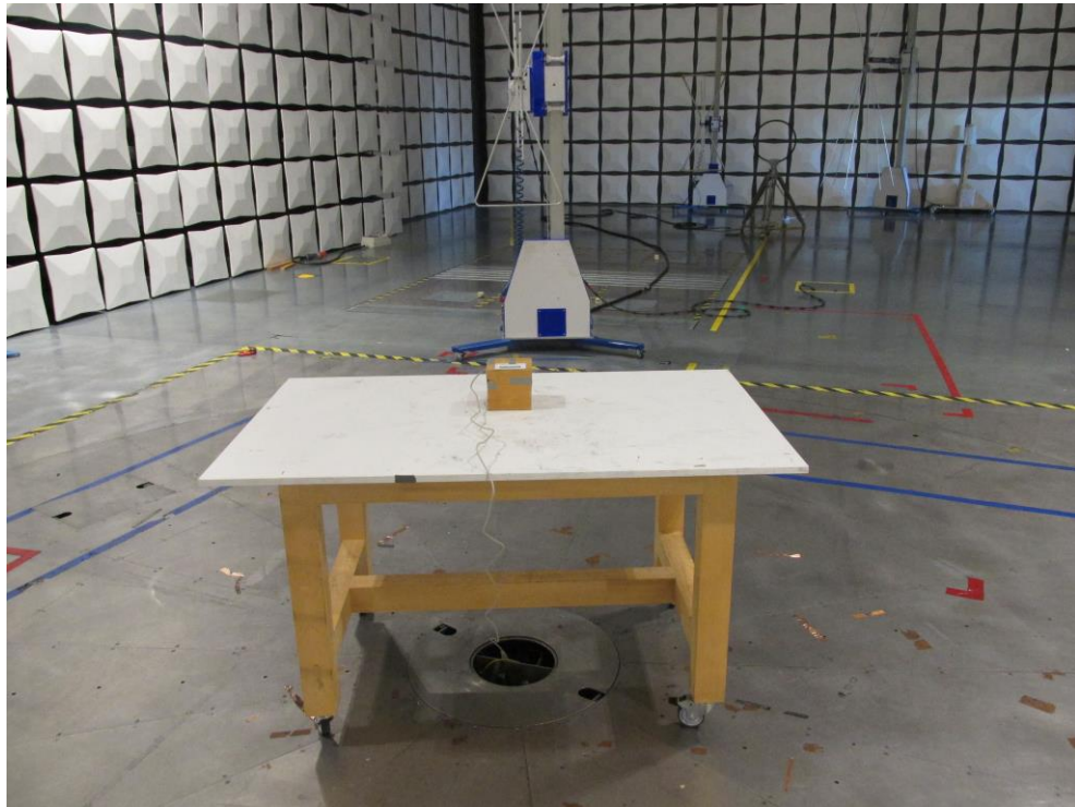
Figure 12 - Test setup for radiated emission
