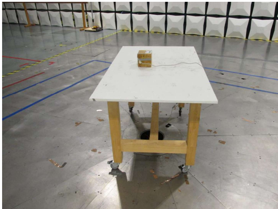
Figure 13 - Test setup for radiated emission
