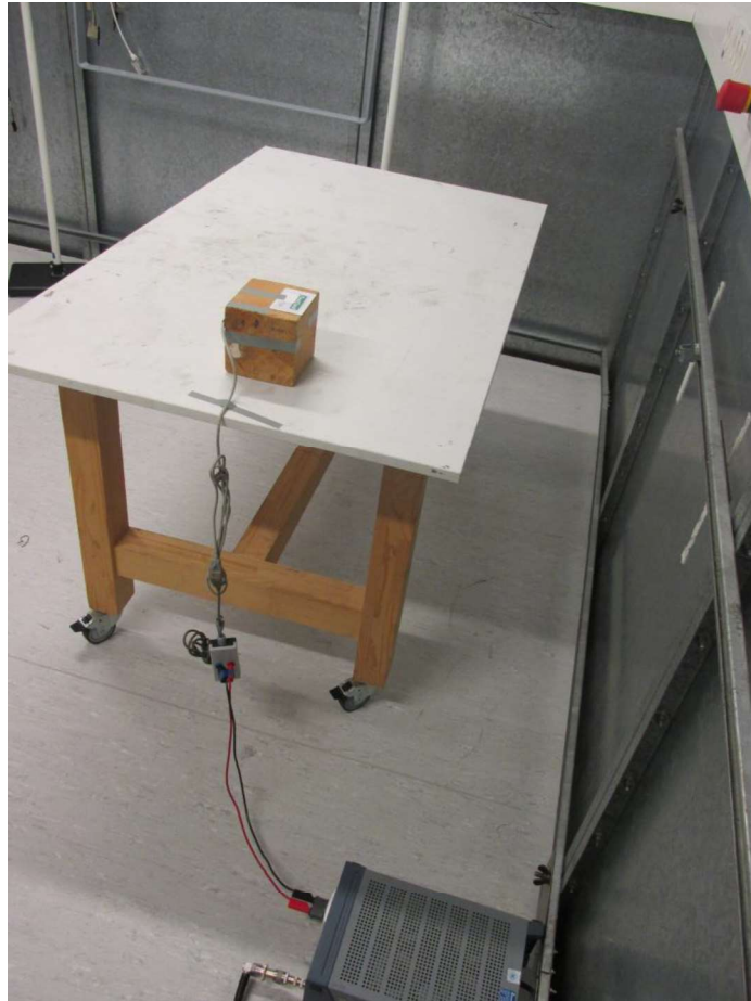
Figure 10 - Test setup for AC Power Line Conducted Emissions
