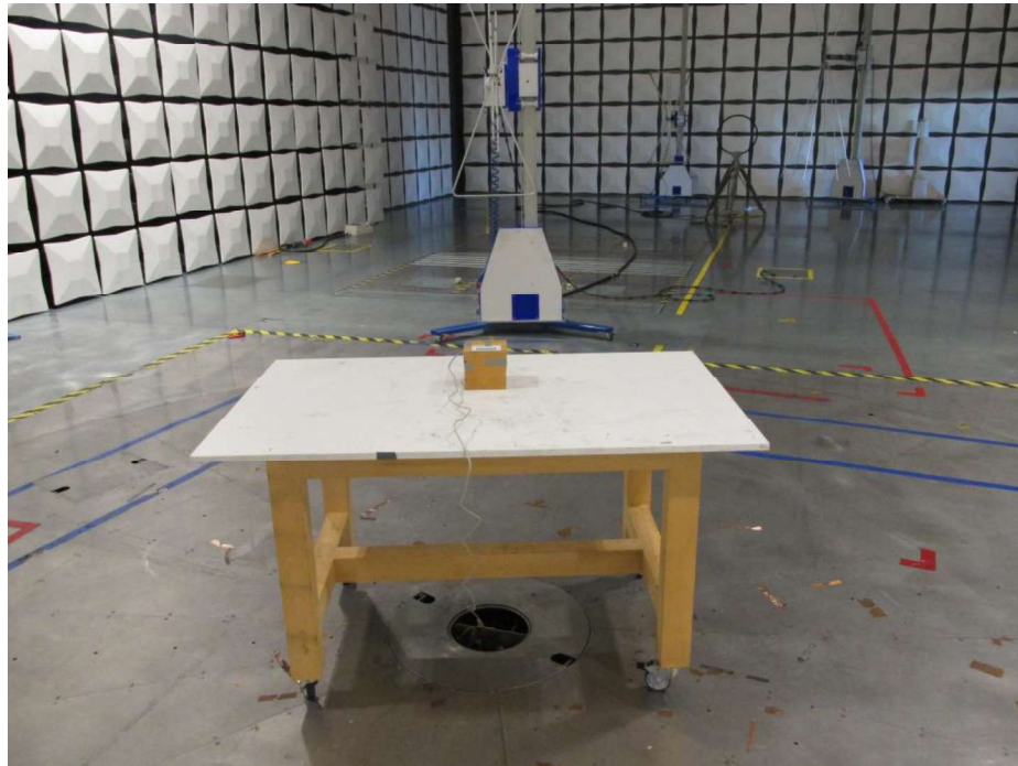
Figure 12 - Test setup for radiated emission
