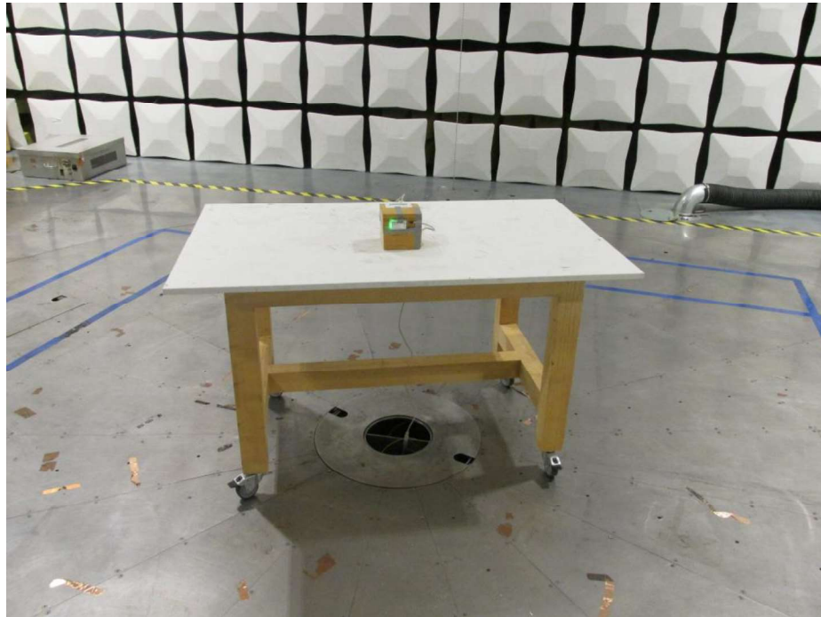
Figure 10 - Test setup for radiated emission
