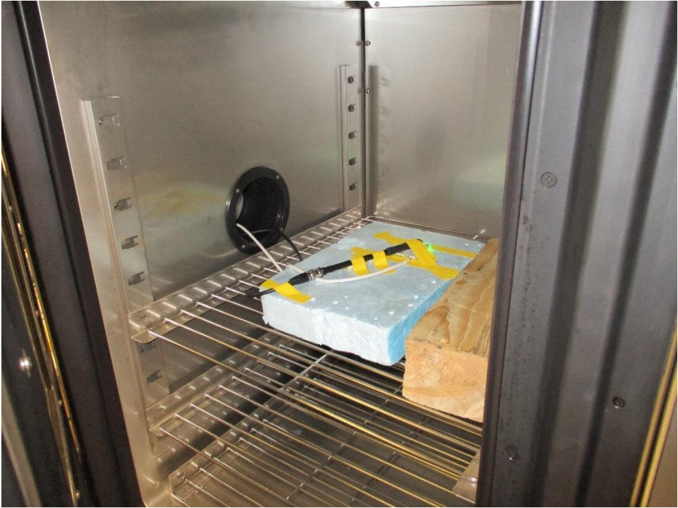
Figure 14 - Test setup for carrier frequency stability
