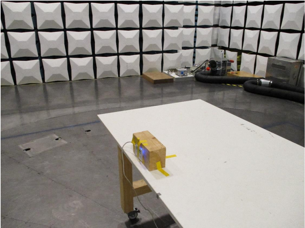
Figure 13 - Test setup for radiated emission 9kHz-30MHz
