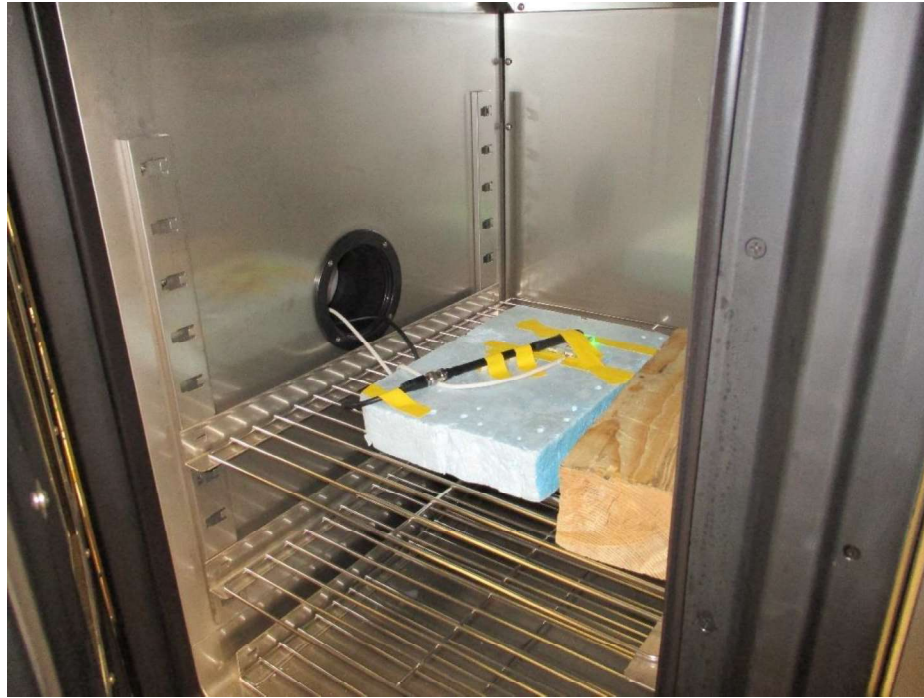
Figure 14 - Test setup for carrier frequency stability
