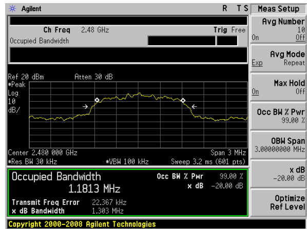
20dB Bandwidth plot on channel 78 (2Mbps)
