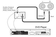
1.Connect the AV cable to the Audio Output Jacks (White Jack=L, Red Jack=R) on DVD player and Audio Input Jacks on the rear of the unit. NOTE:
