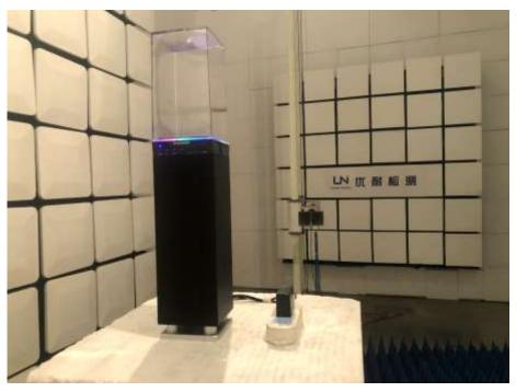
Transmitter Radiation Measurement above 1GHz
