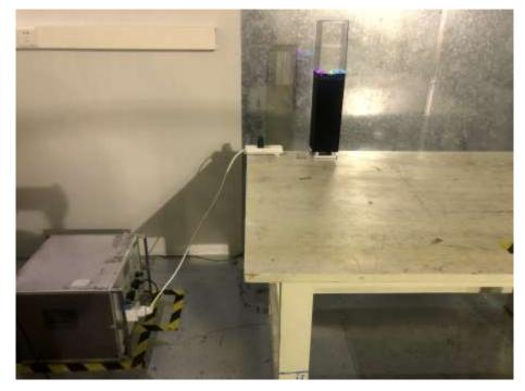
Transmitter Radiation Measurement below 1GHz
