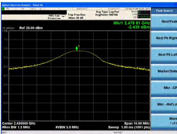
Peak output Power plot on channel 78 (1Mbps)
