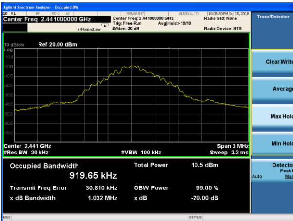
20dB Bandwidth plot on channel 78 (1Mbps)
