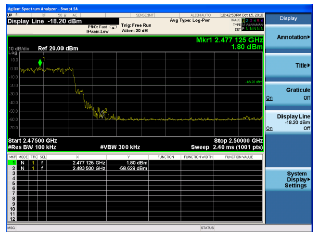
8-DPSK: Band Edge-High Channel (Hopping Mode)
