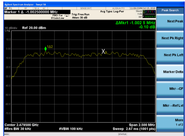
(2Mbps) Channel Separation plot on channel 77-78
