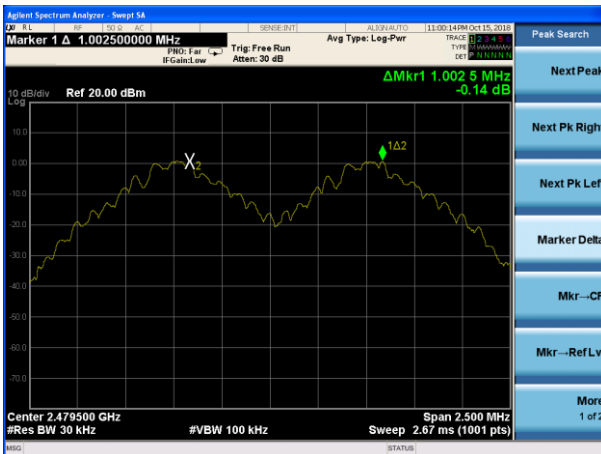
(1Mbps) Channel Separation plot on channel 77-78
