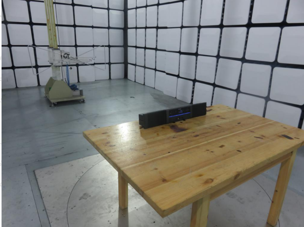
Photo of Radiation Emission Test
