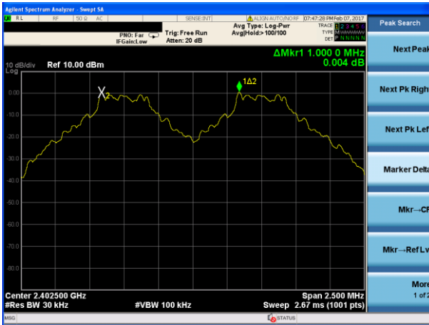
(1Mbps) Channel Separation plot on channel 39-40
