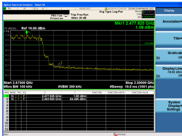
EDR mode ( \pi/4 -DQPSK): Band Edge-High Channel (Hopping Mode)
