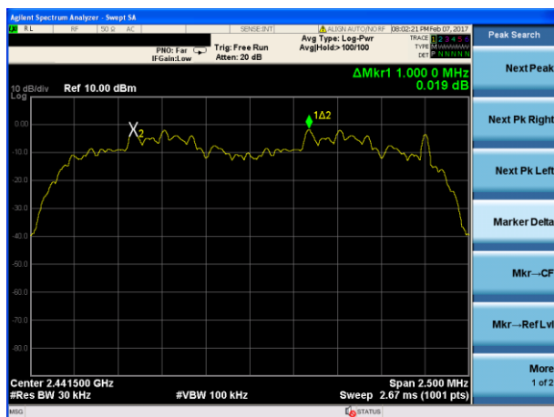
(3Mbps) Channel Separation plot on channel 39-40
