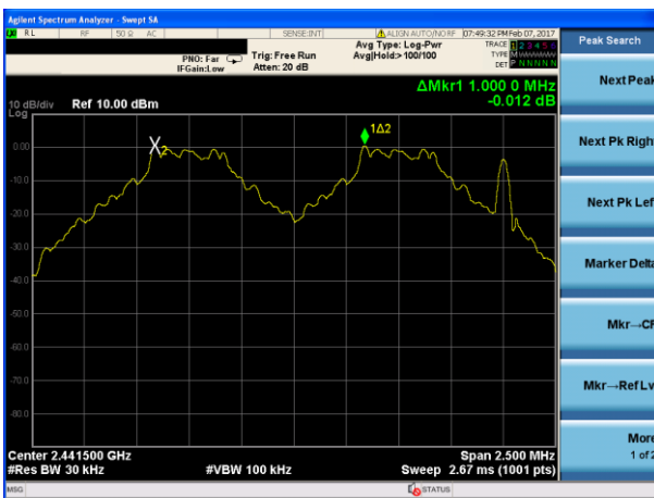
(1Mbps) Channel Separation plot on channel 39-40
