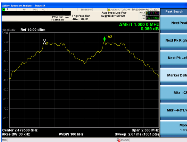
(1Mbps) Channel Separation plot on channel 77-78
