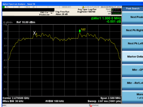
(3Mbps) Channel Separation plot on channel 77-78
