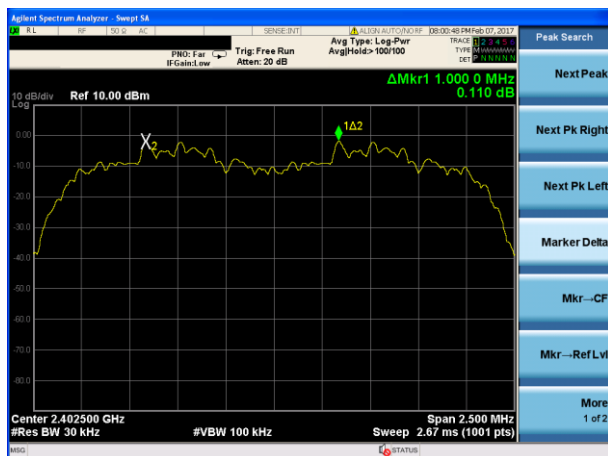
(3Mbps) Channel Separation plot on channel 00-01
