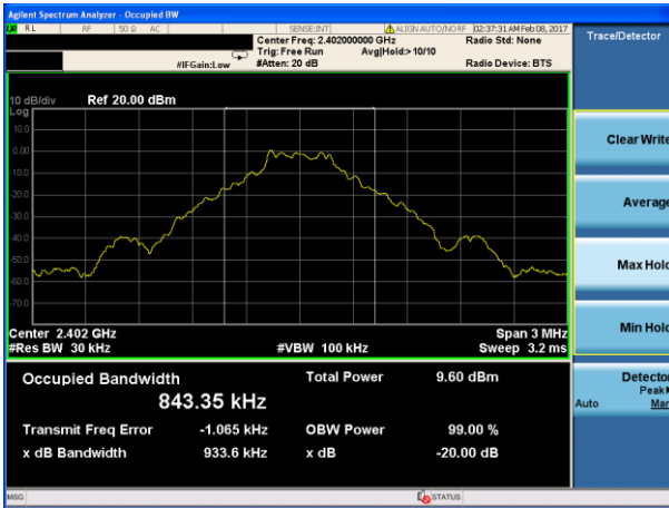
20dB Bandwidth plot on channel 39 (1Mbps)
