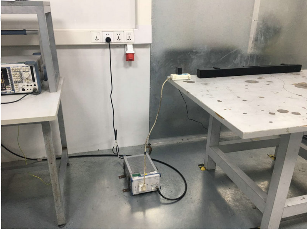
Photo of Conducted Emission Measurement
