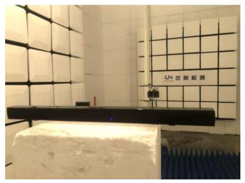
Transmitter Radiation Measurement above 1GHz
