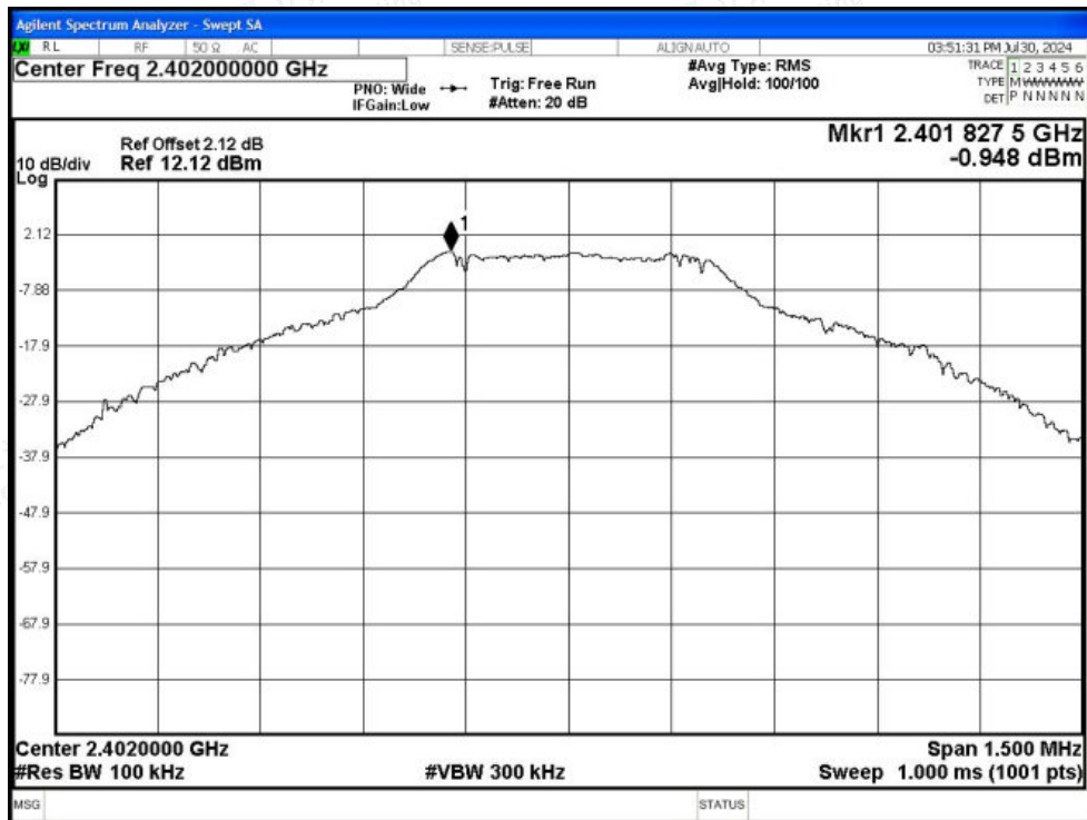
Tx. Spurious NVNT 1-DH5 2402MHz Ant1 Emission
