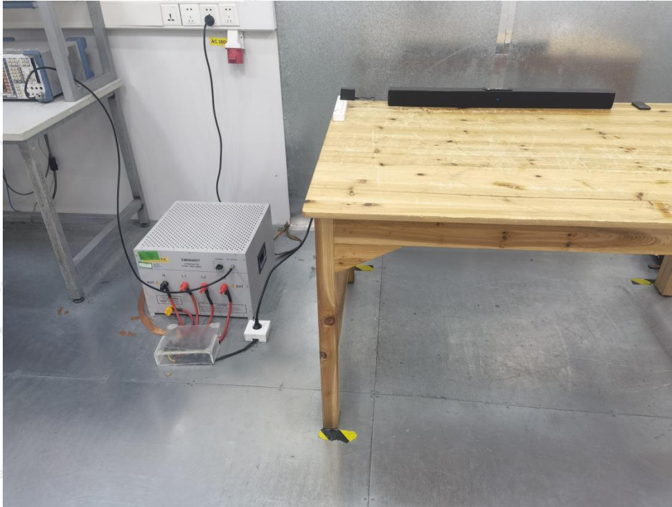
Photo of Conducted Emission Measurement
