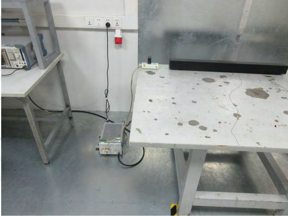
Photo of Conducted Emission Measurement
