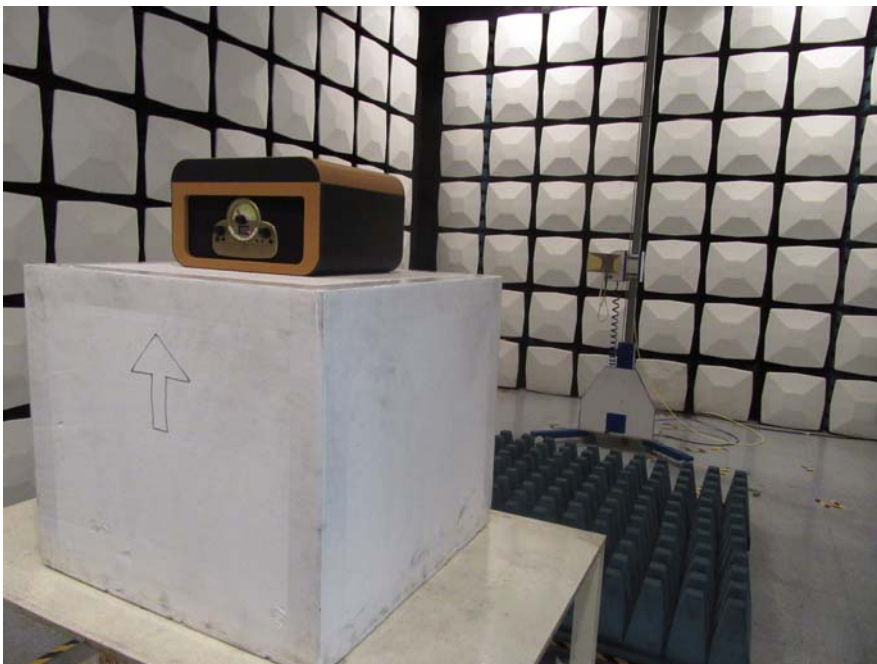
Radiated Emission View (Above 1GHz)
