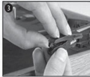
3 separate the cartridge from the socket lightly.
