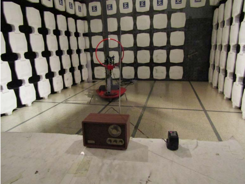
Measurement of Radiated Emission Test Set Up
