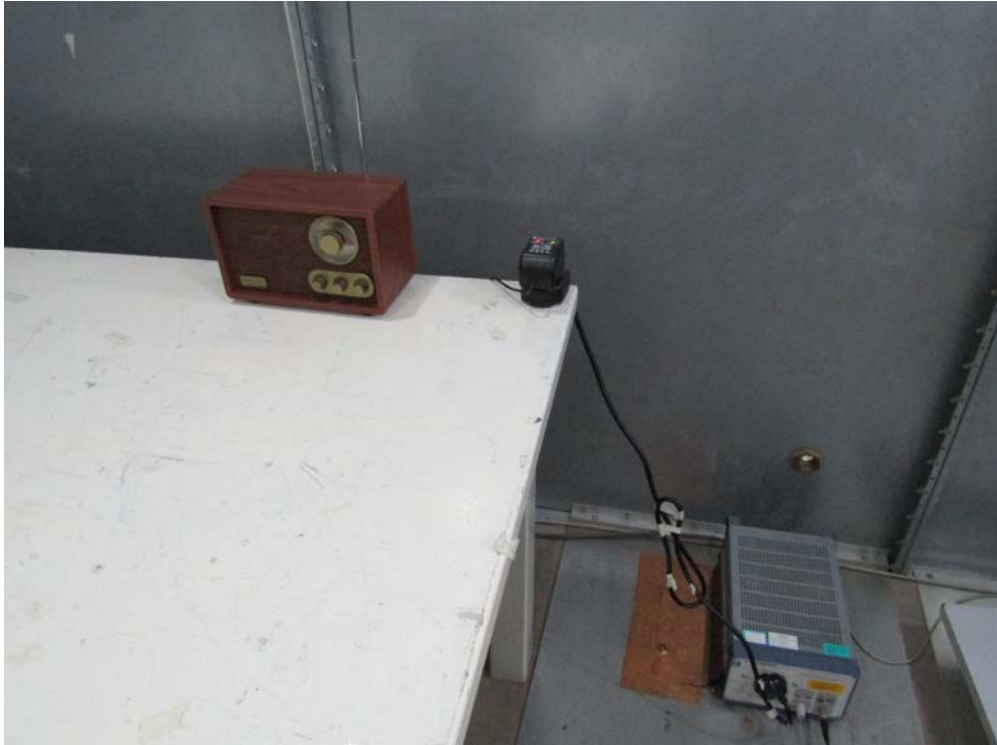
Measurement of Conducted Emission Test Set Up
