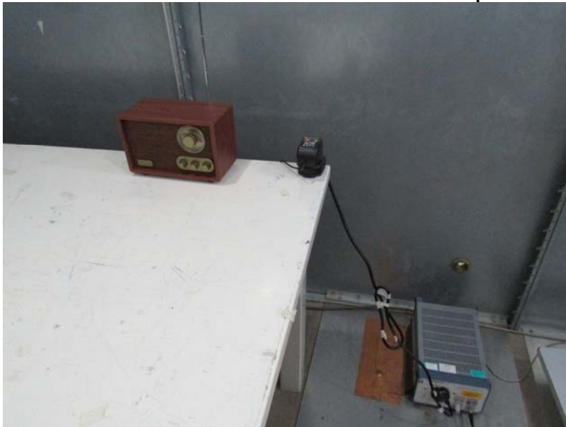
Measurement of Conducted Emission Test Set Up
