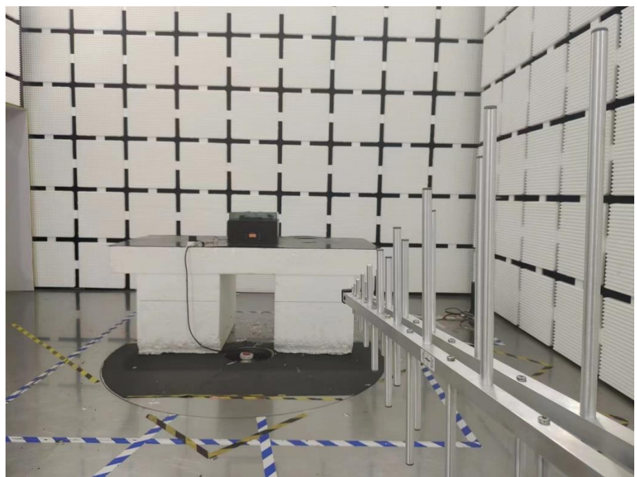
Radiation Emission Test Setup (30MHz to 1GHz)
