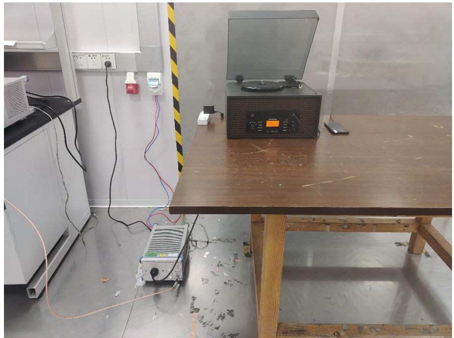
Conducted Emission Test Setup
