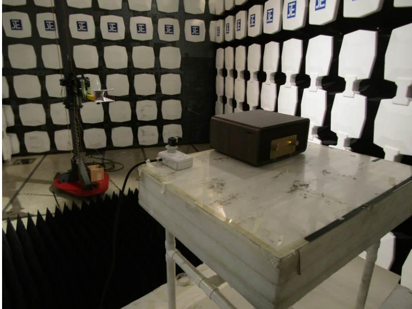
Measurement of Conducted Emission Test Set Up
