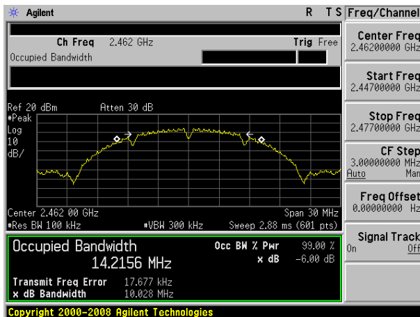
(802.11b) 6dB Bandwidth plot on channel 11
