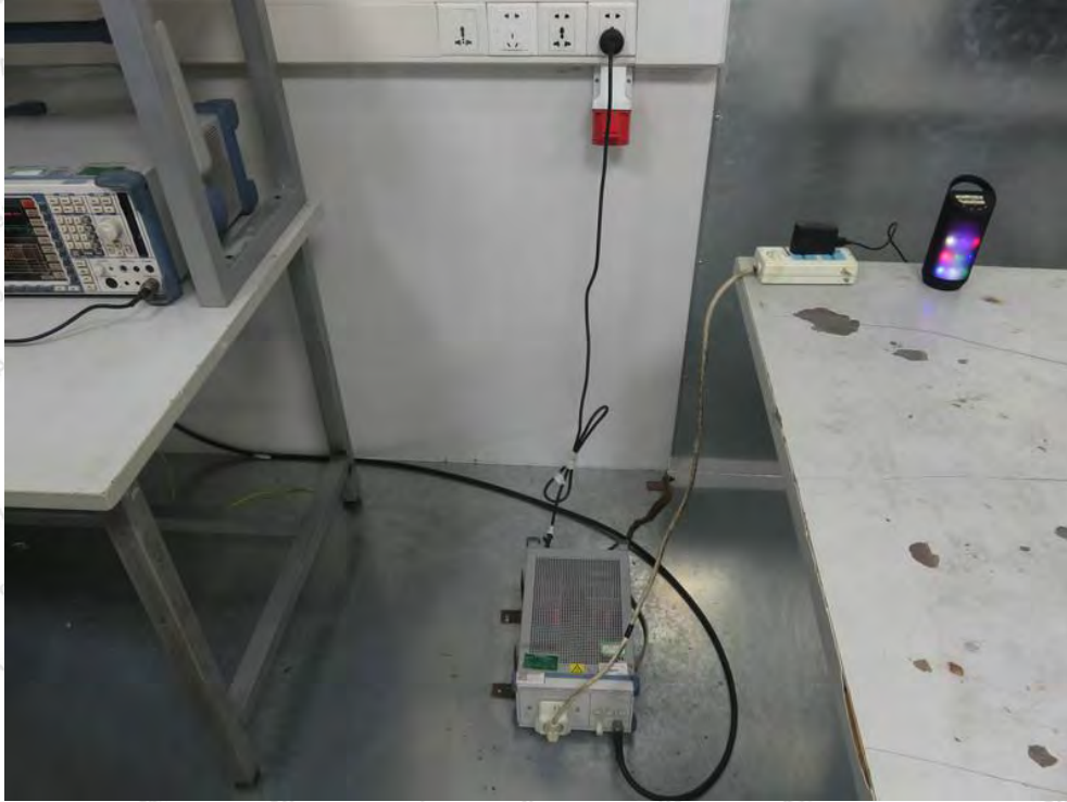
Photo of Conducted Emission Measurement
