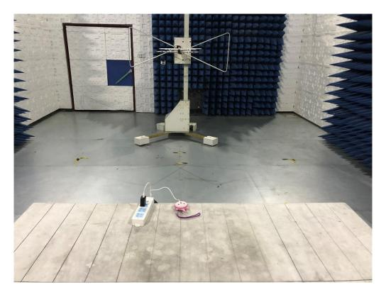
RADIATED EMISSION TEST SETUP ABOVE 1GHZ
