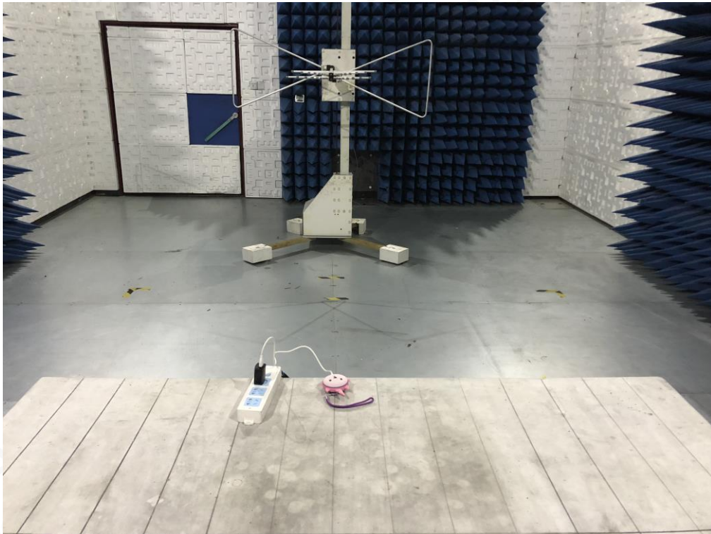
RADIATED EMISSION TEST SETUP ABOVE 1GHZ
