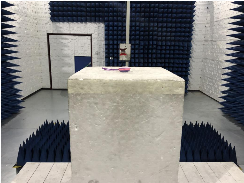
RADIATED EMISSION TEST SETUP ABOVE 1GHZ
