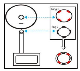
STEP 3: Swivel the horn and the horn rod by reverse direction until they fix each other firmly.
