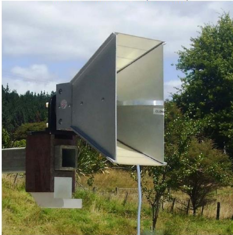
EMCO 3115 Horn Antenna (1 – 18 GHz)
