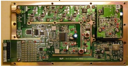
Receiver Assembly w/VCO installed
