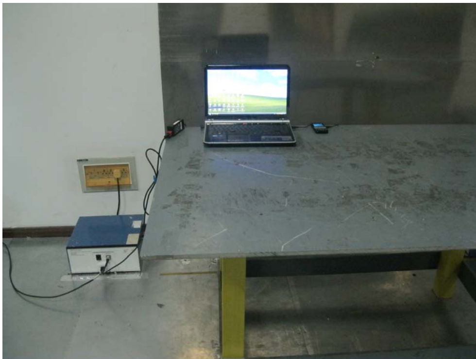
Conducted Emissions Test Setup - Front View
