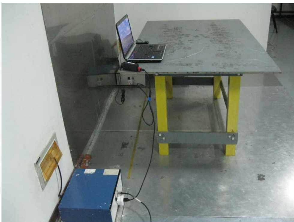
Conducted Emissions Test Setup - Side View
