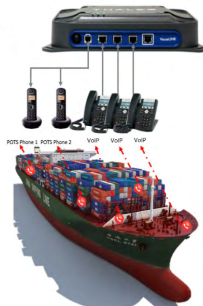
Figure 2-2 Local Communications via PBX Functionality
