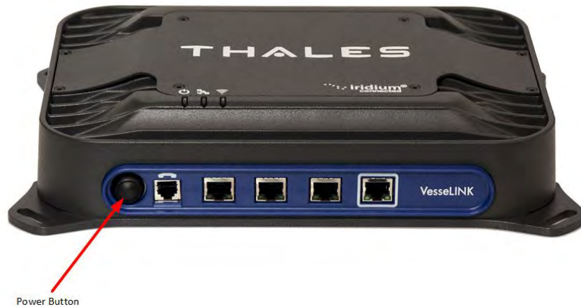
Figure 6-1 Location of Power Button on BDU
