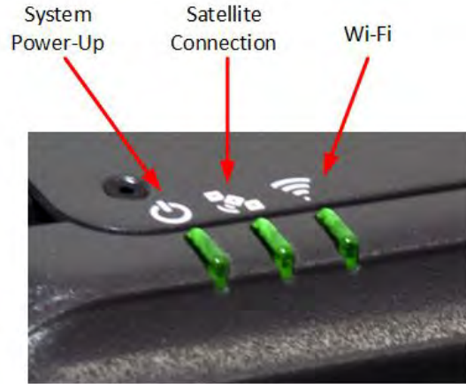
Figure 3-6 System, Satellite and Wi-Fi Status LEDs
