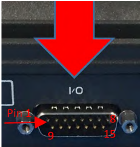
Figure 7-2 GPIO Connector Pin Detail
