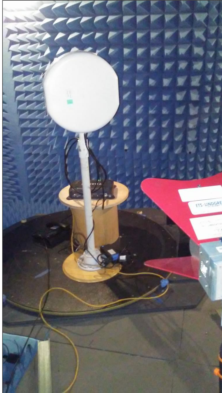
Photograph 2. Radiated Spurious Emissions, Test Setup, Above 1 GHz
