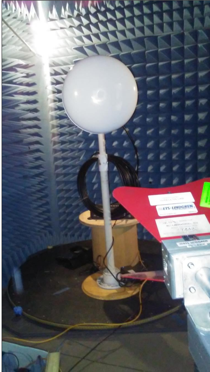
Photograph 2. Radiated Spurious Emissions, Test Setup, Above 1 GHz
