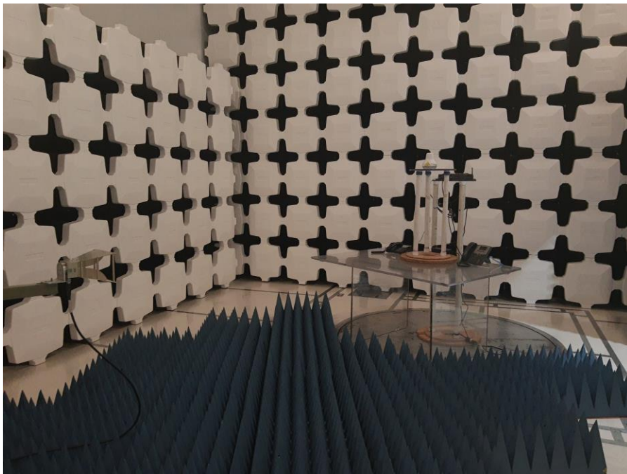
Figure 2: MissionLINK, Radiated Emissions Test Setup, 1-17 GHz
