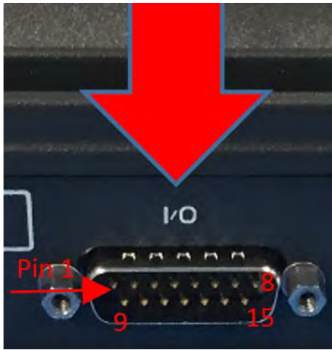
Figure 7-2 GPIO Connector Pin Detail
