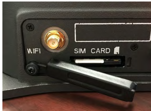
Figure 3-3 SIM Card with Cover Opened
