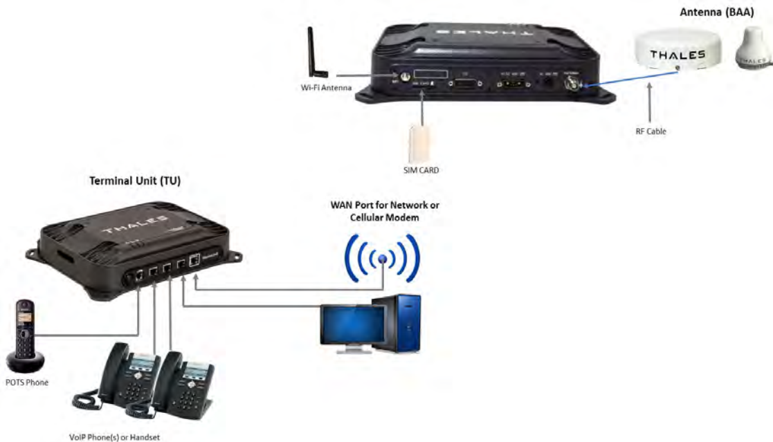
Figure 2-3 MissionLINK System with Connected Hardware
