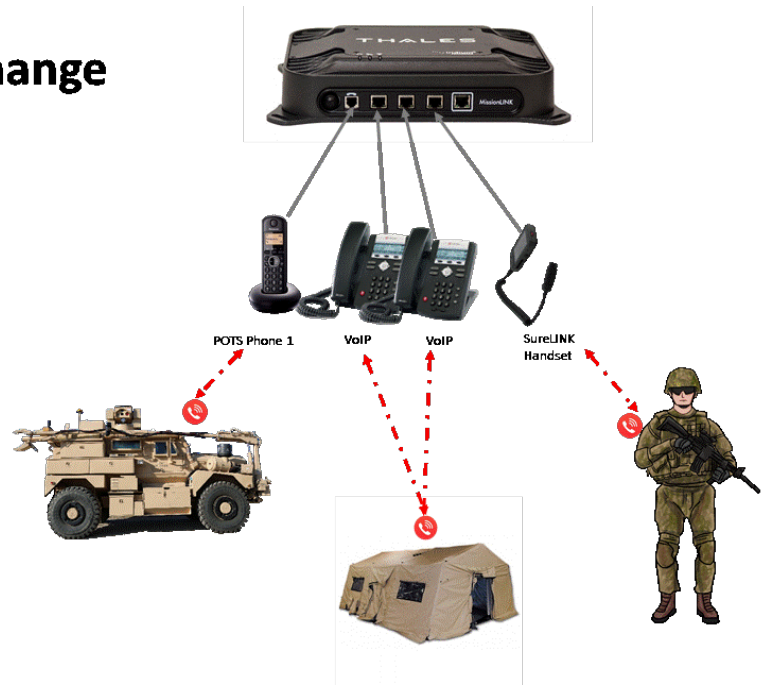
Figure 2-2 Local Communications via PBX Functionality
