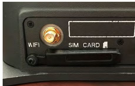
Figure 3-5 Secure the SIM Card Cover
