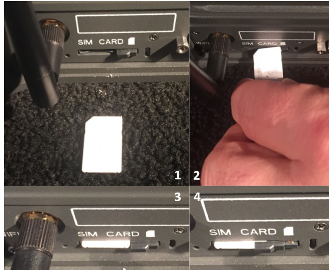
Figure 2-7 Installing SIM Card and Engaging the Lock
