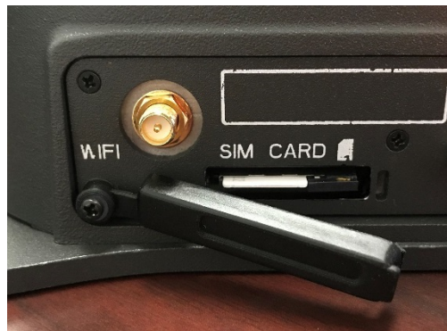
Figure 2-6 SIM Card with Cover Opened
