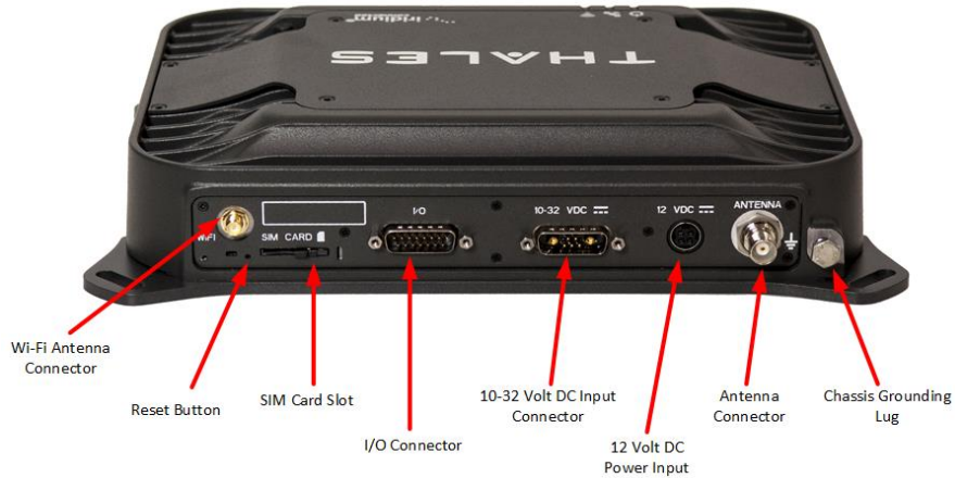
Figure 1-5 Terminal Unit (TU) Back Panel Detail
