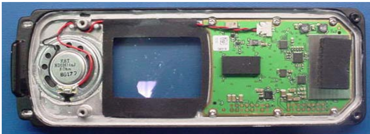
Figure 19 – View of Keypad PWB (4102010-501) onto the Radio Front Cover assembly.
