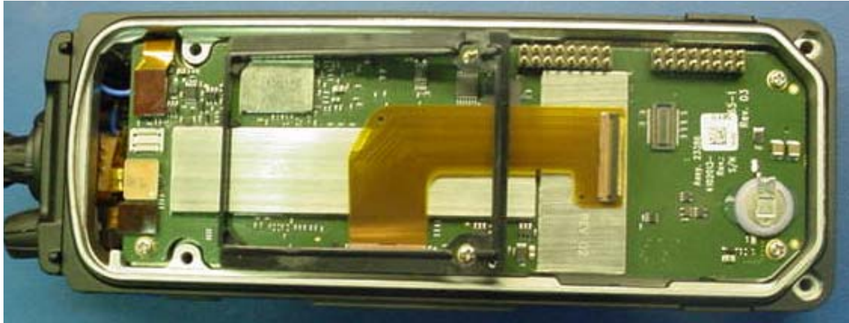
Figure 17 – View of LCD Bracket and Flex Circuit onto the Control PWB (4102013-501)
