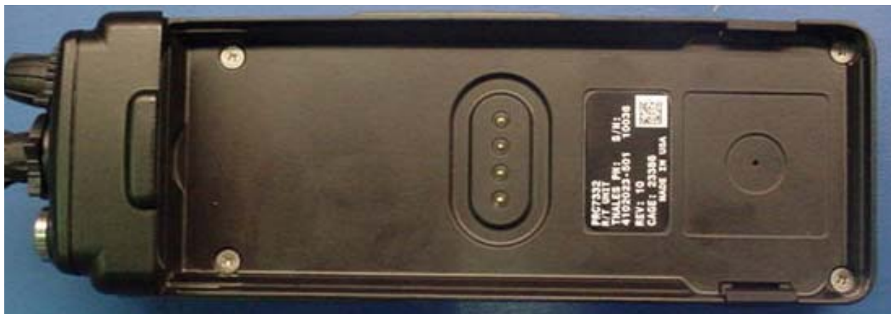
Figure 21 – View of 4 mounting screws to secure the front cover assembly onto the radio chassis assembly.
