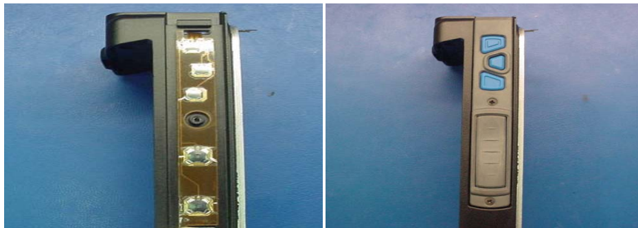
Figure 12 – View of Side PTT Flex Assembly onto Radio Chassis.
