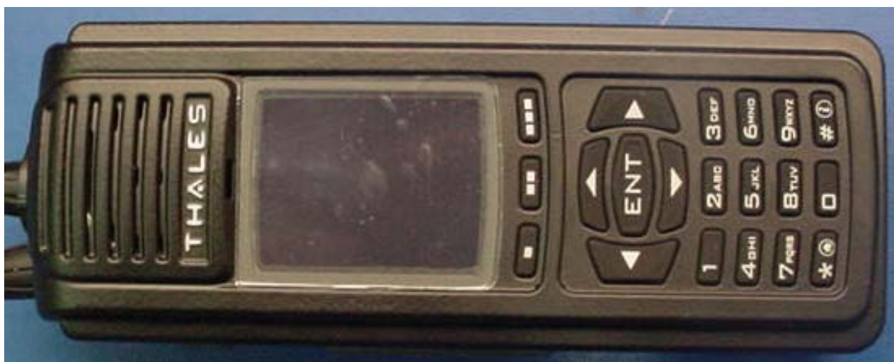
Figure 20 – View of Front Cover Assembly onto the Radio Chassis.
