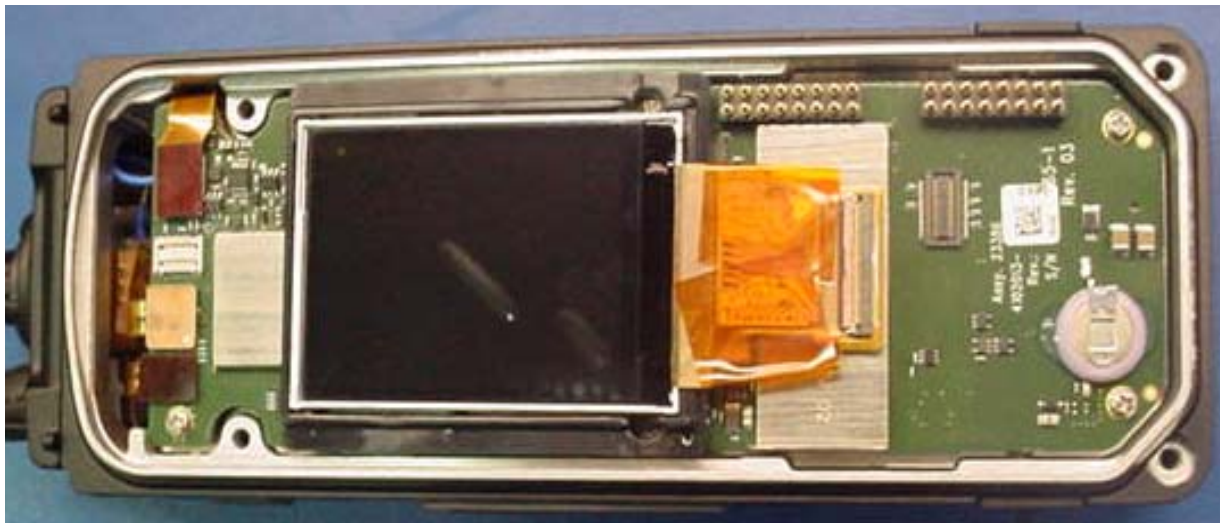
Figure 18 – View of LCD Assembly onto the Control PWB (4102013-501) and connection to LCD Flex Circuit.
