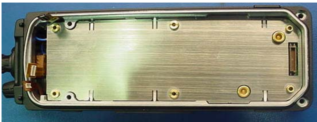
Figure 15 – View of inner shield installation over the XCVR PWB (4102056-501) assembly.
