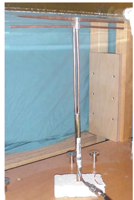
300 MHz Validation Dipole Setup
