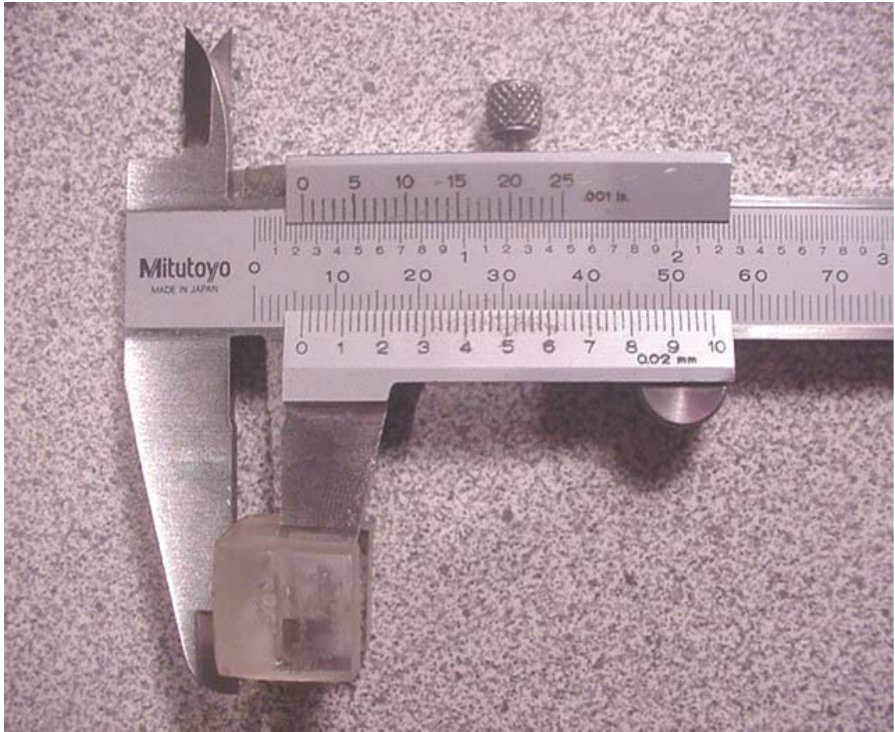
Dipole Spacer Dimension = 6.0mm
