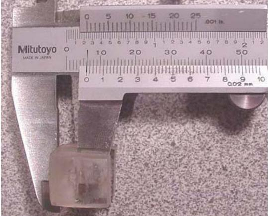
**Dipole Spacer Dimension = 6.0mm**
