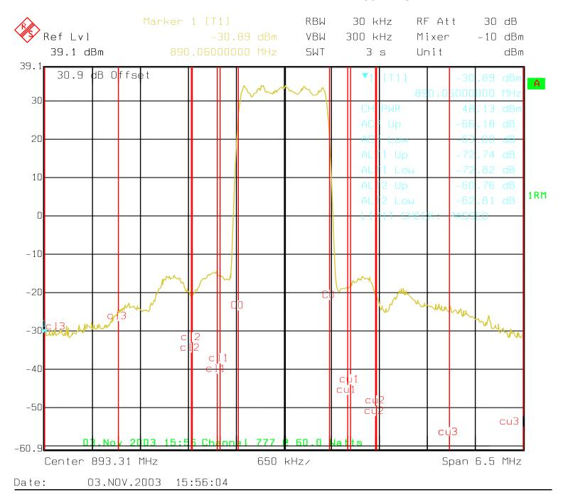
Name of Test: Spurious Emissions at Antenna Terminals
