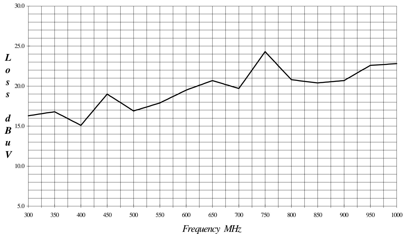
**PREAMPLIFIER EFFECTIVE GAIN AT 3 METERS PA-102 S/N: 1017**
