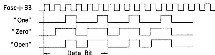
The 'OPEN' state data input will be interpreted as logic low by decoder since the decoder output has only two states.
