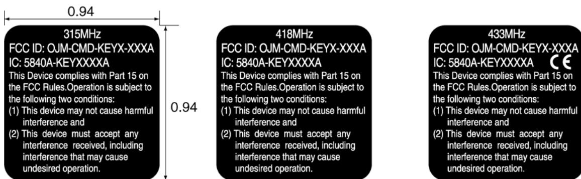
The label is applied to the back of the unit. This is shown below in actual size.
